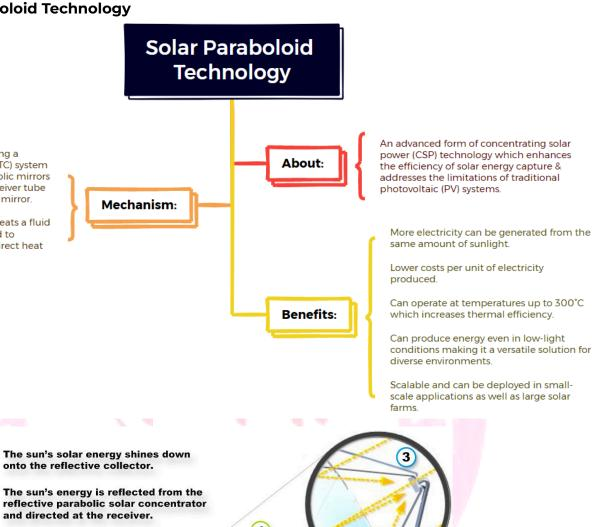
The sun's energy is concentrated 1000 times into the receiver. Various "receiver heads" can be used such as a CPV Multi-junction Solar Cells, Stirling Engine or Ther-
