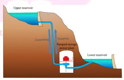
off-peak hours or from renewable sources like solar and wind, it is used to pump water from the lower reservoir to the upper reservoir.
